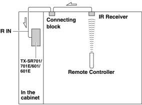
The IR IN input allows you to control the TX-SR701/701E/601/601E from the remote zone (Zone 2) with the remote controller even though the remote zone may be on the other side of the building from the main zone. The diagram below shows how to make the proper connections for the remote zone.
